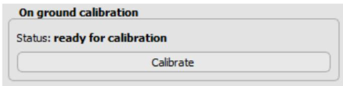
**Step 5:** Hold your *eBee* above the target, making sure that the *multiSPEC 4C* camera is between 50 cm (1.6 ft) and 1 m (3.3 fr) above the target and that no shadows are cast on either the target or the irradiance sensor on the top of the *multiSPEC 4C* camera.
